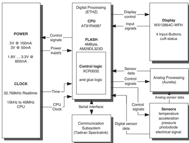
Figure 2: Block diagram of the AMON wearable health monitoring computer.
