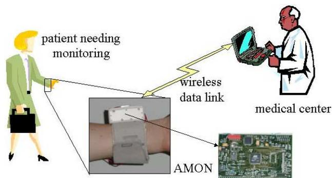
Figure 1: Prototype of the AMON wearable medical computer (box) and its role in the monitoring system.
