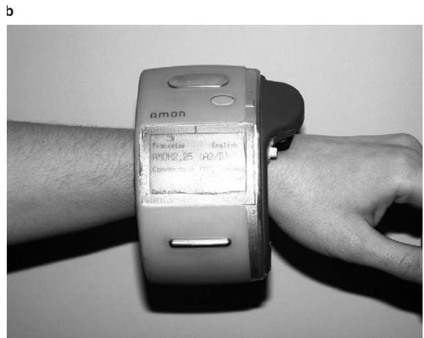
**Figure 2** AMON prototype, mounted on the wrist, positions of sensors are shown. An SpO<sub>2</sub> sensor and thermopile are integrated into the cuff. (a) Cross-section of the first prototype and (b) picture of the second prototype.
