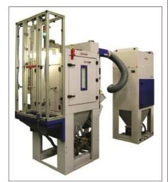
on volumes of components being processed. Each of options involves tight control of parameters such as media type and size, blast pressure and gun angles, surface blast speed and blast nozzle stand-off.
