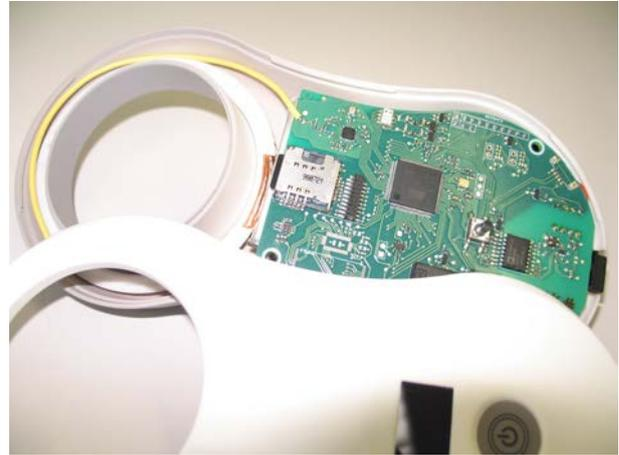
Atmel SAM7X in a battery powered charging and control system for a human medical implant
